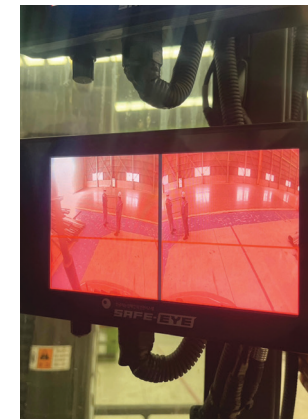
The smart safety system for forklifts
